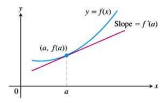
"Close to" the point (a, f(a)), the tangent L(x) = f(a) + f'(a)(x - a) (point-slope form) is a "good" approximation for y = f(x).
