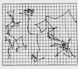
Perrin (1913) 3 colloidal particles. positions joined by straight lines
